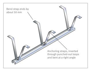
Anchor channel JSA with installed straps.
