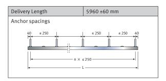
JORDAHL® anchor channels JSA consist of profiles with punched-out loops and associated anchoring straps made of sheet metal strips which are installed on the building site and can easily be bent to shape by hand.
