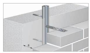
Connection of brickwork support shells to reinforced concrete components with brick tie channel Kt 28/15-D and anchor.
