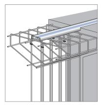
Installation in heavily reinforced elements
