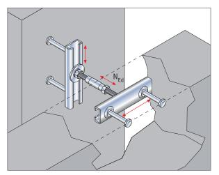
Turnbuckle Connections JSV provide three-dimensional alignment.
