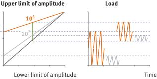
Fatigue resistance at lower limit of amplitude = 0
