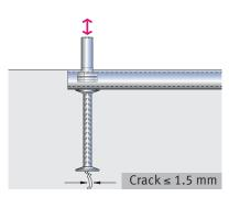
JXA-PC: maximum reliability for high loads and large cracks.
