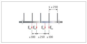
Load arrangement, load pairs.
