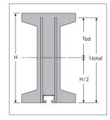
The reinforcing bar anchors must be anchored with anchoring length lbd in the component compression zone. The anchoring length is calculated from half the component height plus anchoring length lbd and must be specified with the order.
