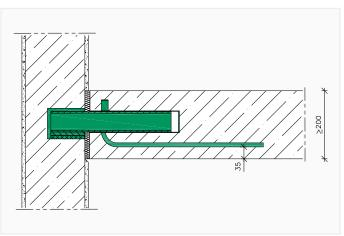
SINTON® HQW 60x60 – Installation for a slab thickness of 200 mm
