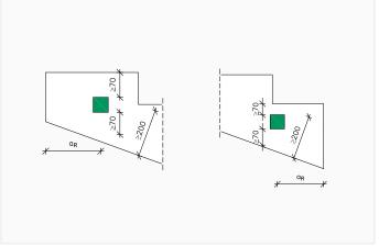
SINTON® HQW 60x60 – Installation in spiral staircases
