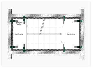
SINTON® HQW in a landing, joint insulation with SINTON® TSP
