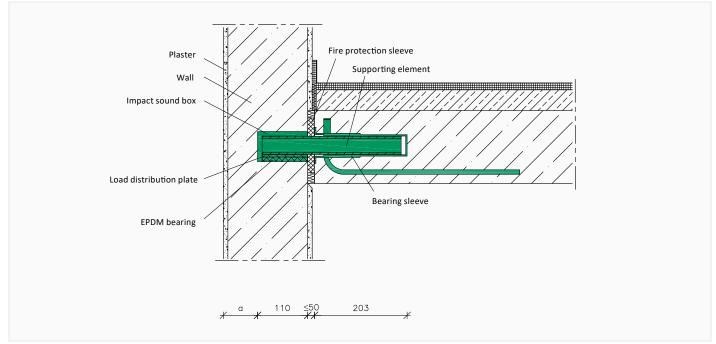
SINTON® HQW fire protection – to meet the requirements for enclosing walls in terms of the fire protection, a clearance (a) of a  $\geq$  40 mm must be maintained.
