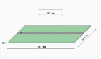
SINTON® ZB dimensions – configuration with linear bearings
