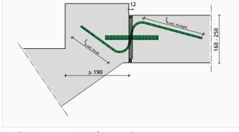
Side view of SINTON® HT-V
