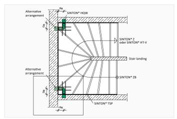
Arrangement of the elements in stair cases – use of HQW with  ${\tt SINTON}^{\scriptsize \textcircled{\tiny B}}$  TSP
