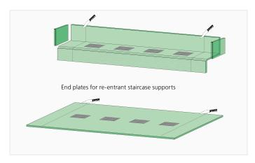
If necessary, the elements can be cut to length with a knife to match the width of the staircase
