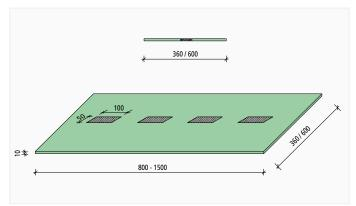
SINTON® ZB dimensions – configuration with single bearings
