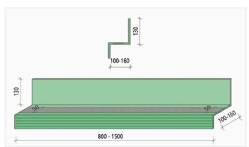
SINTON® Z dimensions - configuration with linear bearing
