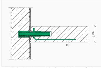
SINTON® HQW 60x40 – Installation for a slab thickness of 160 mm
