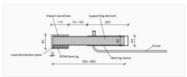
Product cross section SINTON® HQW 60x60 – example with joint width of 120 mm
