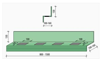
SINTON® Z dimensions - configuration with single bearings
