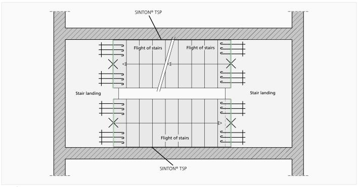
Use of SINTON® HT-V in a landing in combination with SINTON® TSP
