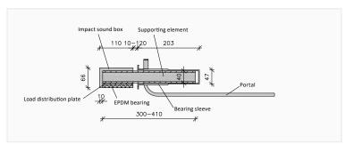
Product cross section of SINTON® HQW 60x40 - example with joint width of 15 mm with TSP
