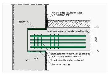
Installation cross section SINTON® X
