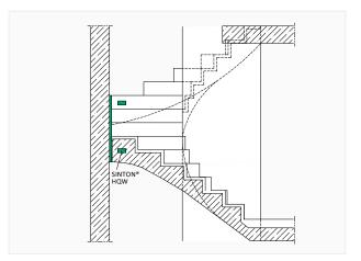
Use of SINTON® HQW in a half-spiral staircase, joint insulation with SINTON® TSP
